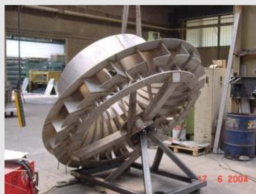
BSK®-surface aerator under manufacturing in the Biogest-workshop.
