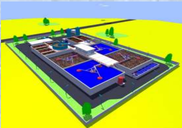
Illustration no. 4: Pre-designed OTR-treatment system for an industrial field in the South of China. The hydraulic connection load is 10,000 m 3 /d and the organic pollution reaches up to 80,000 p.e.
