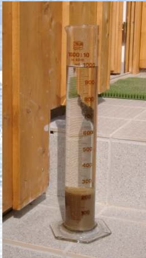
Photo no. 7: The test-cylinder is demonstrating one of the typical process-steps of the OTR-operating: settling has already be finished, so that the clear water could be discharged by the decanter. Settling and effluent discharge take place under perfect conditions - in contrary to conventional clarifiers, in which settling and overflow has to be managed simultaneously.
