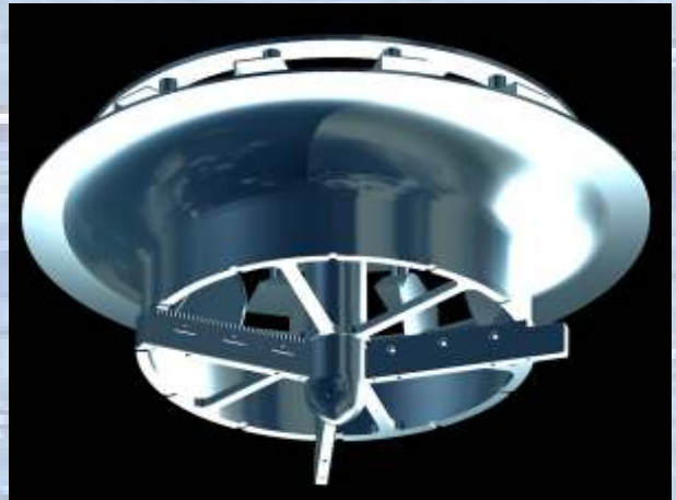
Illustration no. 3: BSK-Turbine with a solids macerator. Preferably to be used in smaller OTR-plants in order to avoid a screen for solids-removal.
