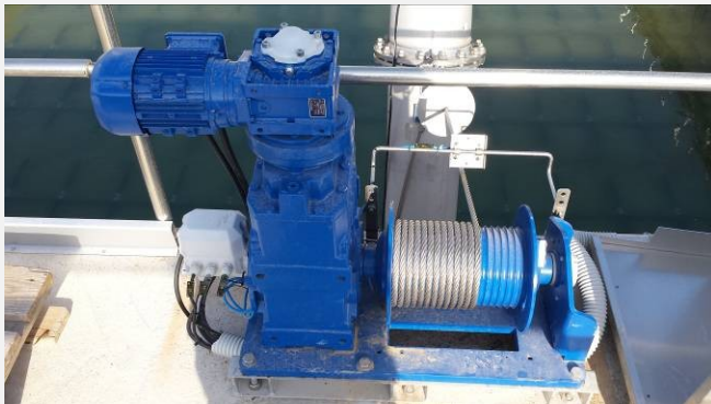
BSK®-decanting winch including drum, electrical drive and limit switchbox
